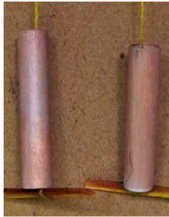
Second coat of toilet bowl cleaner dried. At this stage it doesn't look like much has happened but be patient, it gets better with time and weather
