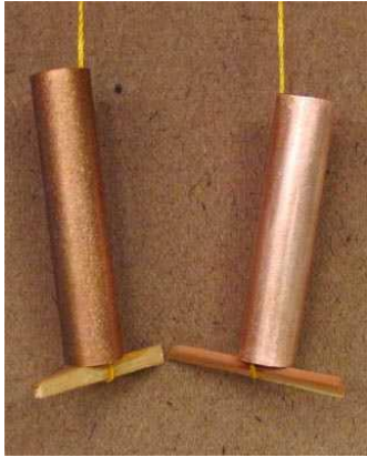
Cleaned and ready for the process. The tube on the left was sanded with 150 grit sand paper while the right hand tube was cleaned with steel wool
