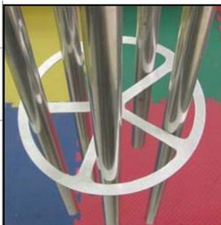
The strike energy from a radial striker is better distributed among the chimes in the set than it would be from a single circular shaped striker. Each chime receives less energy because of this distribution and produces a somewhat muted sound. Therefore, a more robust strike is required to increase the loudness of the chimes.
