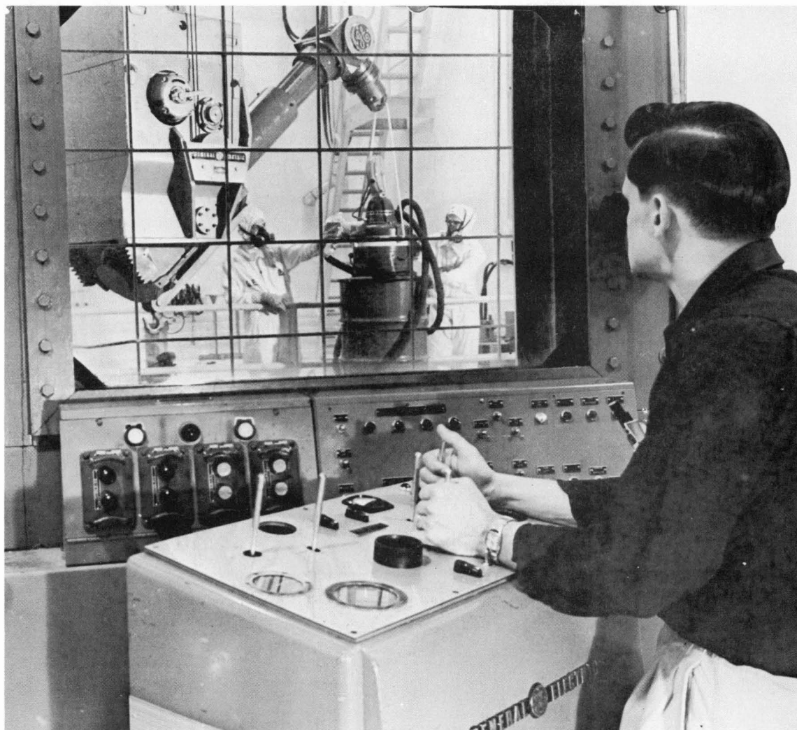
Figure A-11 - View from Hot Shop gallery showing use of remote manipulators combined with limited manual operation.
