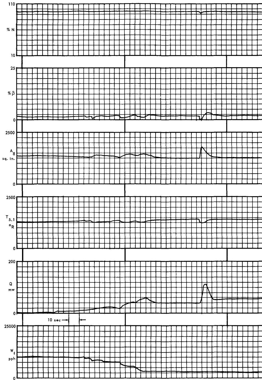
Fig. 7.37a—Analog computer study of power transfer CHO to NHO during ITS hot day conditions
