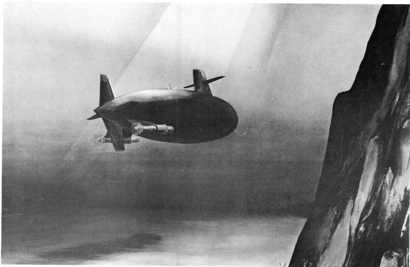
Fig. 11.4—Installation of 601B power package on a submarine
