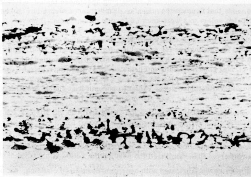
Fig. 5.19—Porosity in the core-cladding diffusion zone as observed in uncracked material near the center of the specimen
