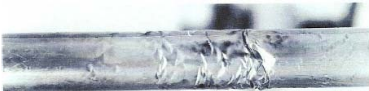
Figure 2-9 Insulation Liner Showing Wrinkling
