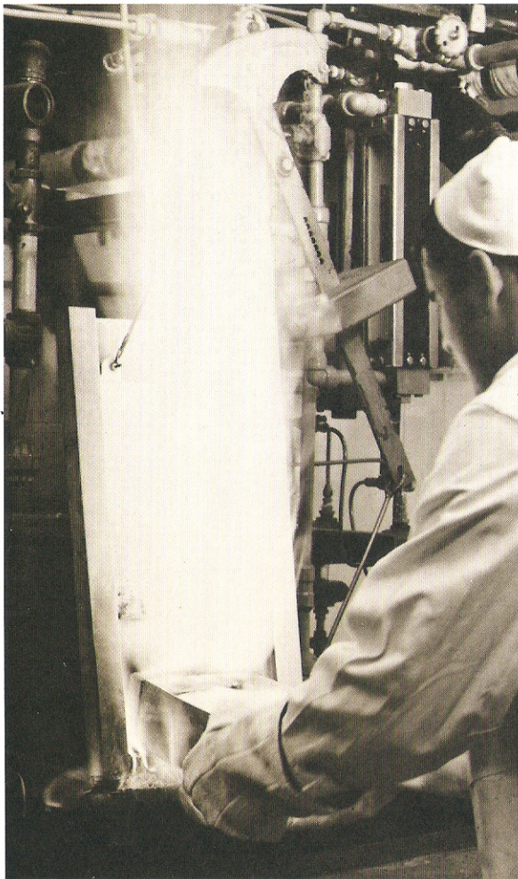
The "flame curtain" automatically flares up when sintering door opens to prevent contamination of the pure hydrogen atmosphere in this ceramic sintering furnace.
