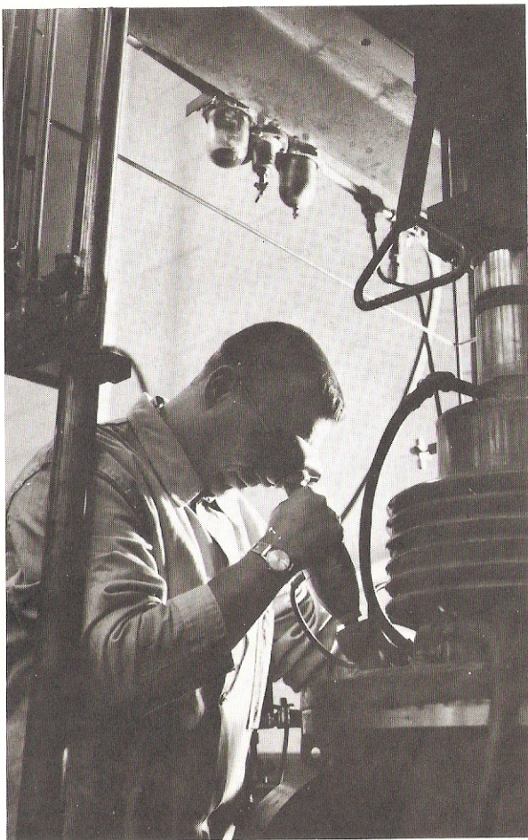
Metallic and non-metallic materials are densified by vacuum hot pressing, a process which eliminates atmospheric contamination and also removes volatile impurities. Densities up to 100 percent of theoretical are obtained.
