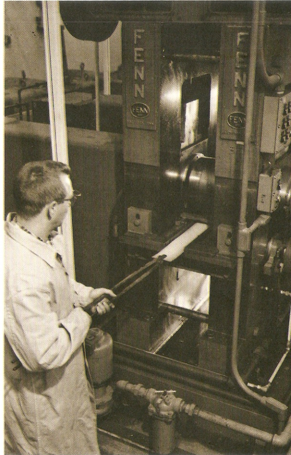
Cold-rolling ductile tungsten alloy sheet. The rolling mill is equipped with special controls as well as solid tungsten carbide rolls.
