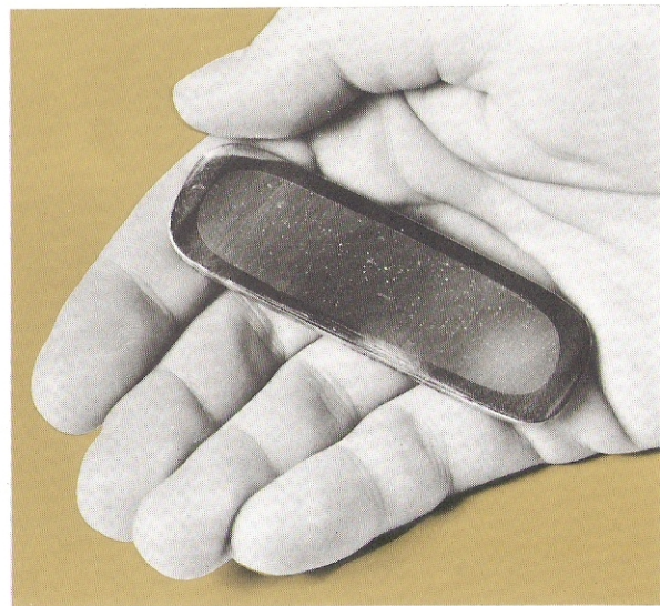
Cross section of a co-extruded reactor control rod; cladding — Inconel 600, core — dysprosium oxide dispersed in nickel.
