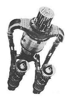
Several Heat Transfer Reactor Experiments (HTRE) were conducted at the Government's National Reactor Testing Station, located in a remote part of Idaho from 1955-1960. The equipment required for these tests was huge, heavy...and expensive. No effort was made to minimize their size for application in airframes.
