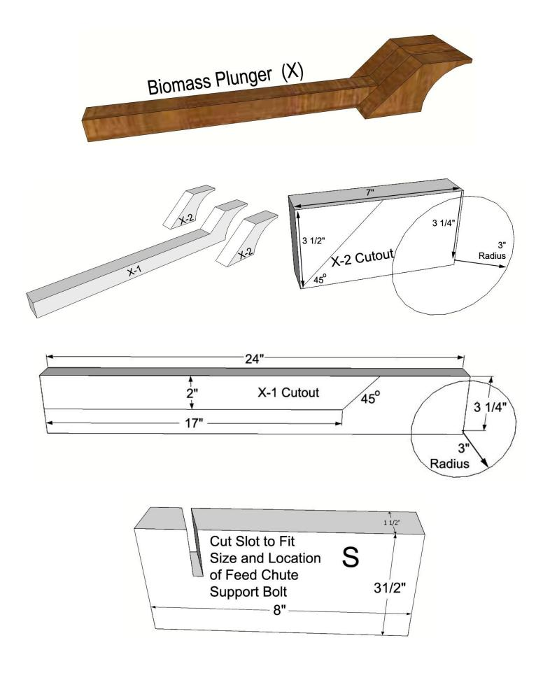
The dimensions are based on a standard lumber size of 3  $\frac{1}{2}$ " wide X 1  $\frac{1}{2}$ " thick material, and 5  $\frac{1}{2}$ " wide X 1  $\frac{1}{2}$ " thick material. The grinder can be constructed using softwood.
