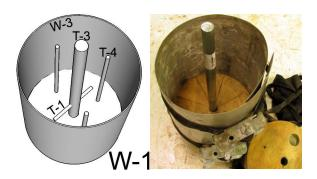
Loosely fit the second strap clamp to the top of the cylinder. Tighten the lower clamp so the sheeting is pulled tight around the bottom end cap. Lightly coat the inside surface of the cylinder with oil or light grease. Fill the mold with concrete containing aggregate to about 1 inch from the top.
