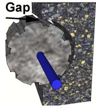
cup for biomass to enter into the grinding space. This adjustment may vary a little depending of the type of biomass. Adjust until you are happy with the grinding output.
