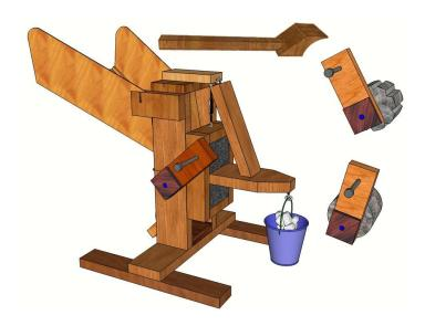
The biomass grinder was designed to grind dry biomass and to accomplish several goals. The objectives were the flexibility to grind a wide variety of dry biomasses, low-cost, easy to build using mostly hand tools, easy to operate, easy to maintain and require no welding.
