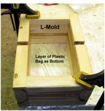
After the no teeth grinding head (NA) has cured for a few days, wrap it tightly in plastic and insert it into the two slots in the L-Mold. Fill the mold with concrete and jiggle to remove air bubbles.
