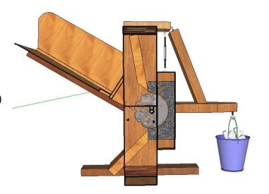
Temporarily attach the feed chute support brackets (S) to the top of part (E).
