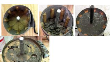
Remove the cylinder when you are comfortable that the concrete has cured sufficiently to be able to wire brush the teeth to expose the aggregate. Do not wire brush the V section of the teeth. Again, keep the end caps in place for about 24 hours until the concrete has cured enough to safely remove them without damaging the edges. Again, cover with a wet cloth and plastic and keep wet for curing.
