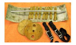
Insert T-1 pin in the center of shaft T-3, and push T-3 through the end cap V-1 so the radial lines are visible from the inside of the mold.
