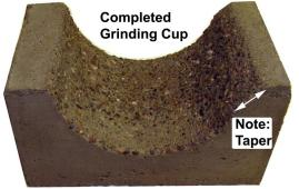
Remove the four sides of the mold when you are comfortable that the concrete is firm but soft enough to scrub to expose the aggregate. Make certain that you scrub from both sides toward the center so as not to damage the edges.
