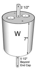
Double check to make certain that the end caps are perpendicular to the shaft and that the end caps are evenly inserted into the very ends of the cylinder. They should not be pushed beyond the end of the cylinder. The objective is to have the ends parallel to each other and perpendicular to the shaft.
